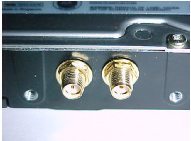
Figure 1: SMA Connectors Mounted on Drive Case
