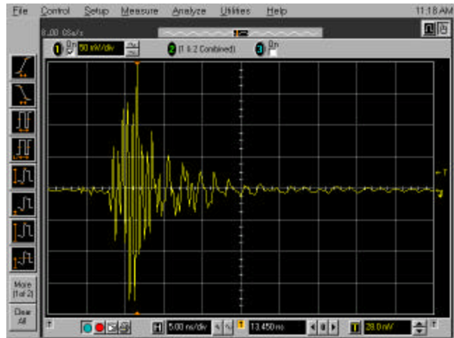
Figure 12: Loop Pickup from Copper Tape Spark Gap
