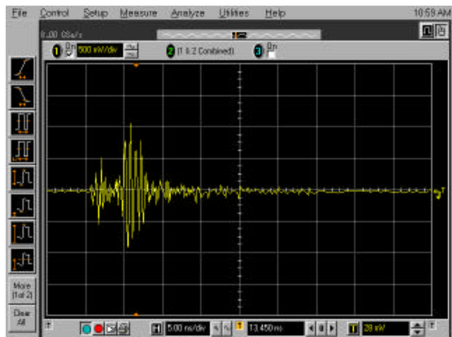
Figure 10: Loop Output from Discharge to Top of Drive Enclosure
