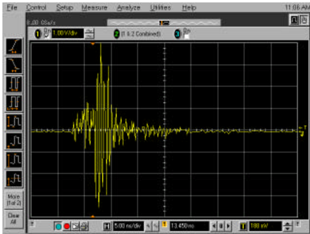
Figure 11: Loop Output from Discharge to Edge Near the SMA Connectors.
