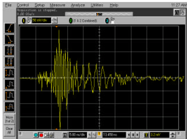
Figure 13: Loop Pickup from ESD Simulator Self-Discharge
