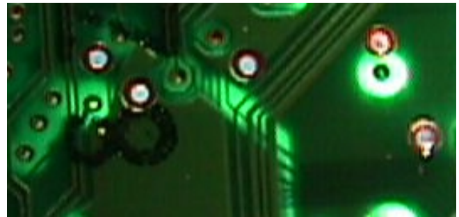
Figure 10. Example of Paths Crossing Break in Ground Plane
