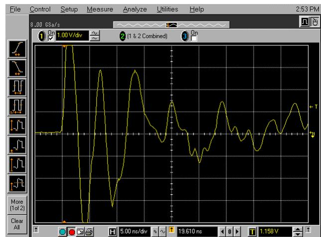
Figure 5: Field Strength Resulting From Disk Array Insertion
