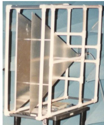
Figure 1: TEM "Time Domain" Antenna
