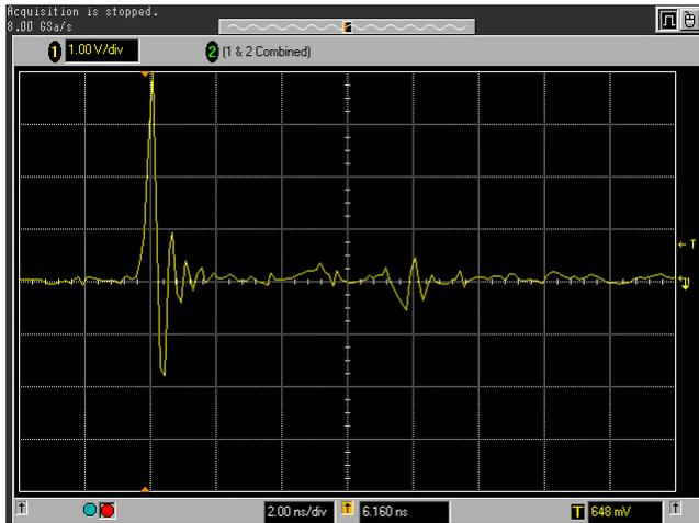
Figure 2: Response of TEM Antenna to Small Metal ESD
