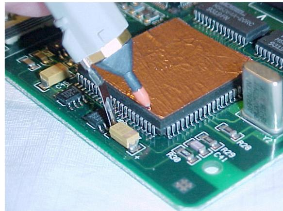
Figure 6. Capacitively couple measurement.[2]
