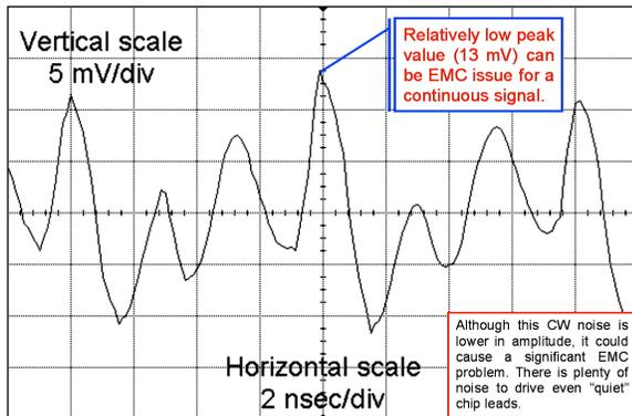
Figure 5. Example of a typical EMC problem.[2]
