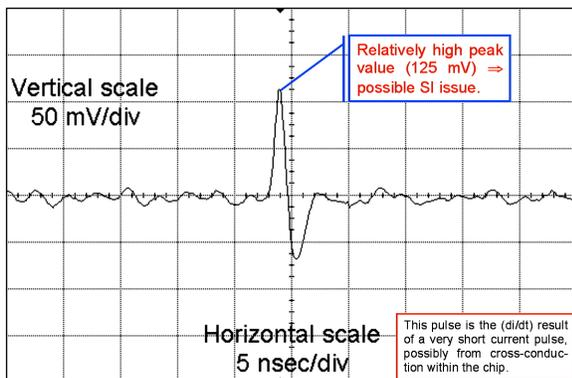
**Figure 4. Example of a typical SI problem.[2]**
