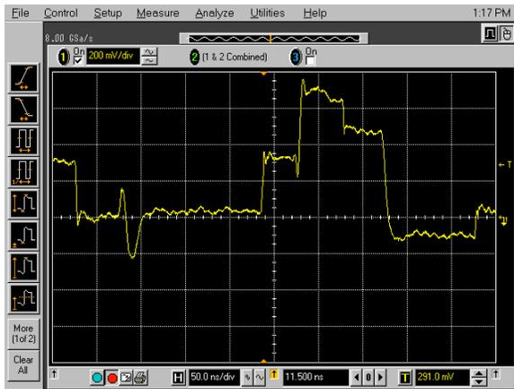
**Figure 7. Measured voltage on copper foil for modem IC.[2]**
