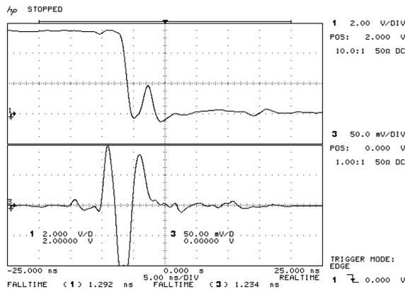
**Figure 3. Loop output, lower trace, and IC output pin, upper trace, show the problem.[2]**
