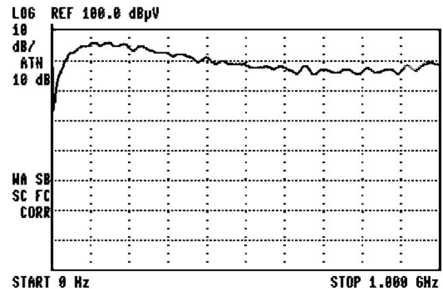
Plot 13: Loops Separated by 3 mm (1/8 Inch) Air
