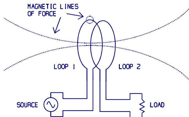
Figure 1: Transmission Between Loops [2]
