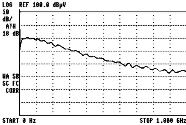
Plot 9: Shielding for Electronics Sample "B"
