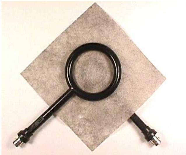
Figure 3: General Shielding Measurement Setup [2]
