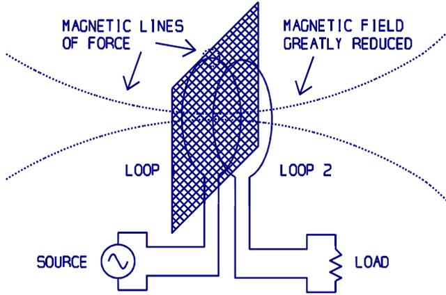
Figure 2: Shielding Material Placed Between the Loops [2]
