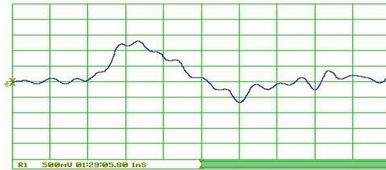
8" disk, 1kV. Peak I is over 10A
