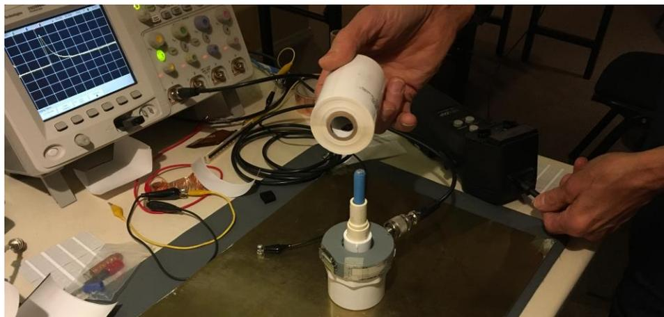
**Figure 2.** Measuring the Discharge Current from the Print Media
